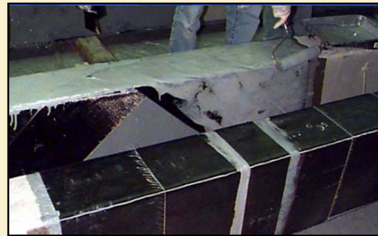
Photos show development and testing of methods of applying carbon fiber in UK labs.
